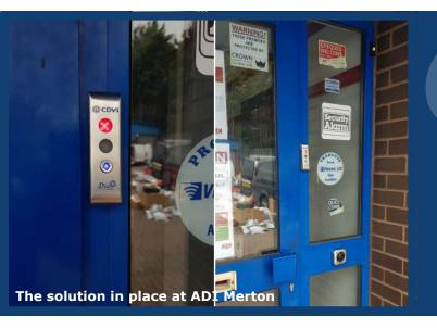
"In order to operate safely during the COVID-19 pandemic and easing out of lockdown, we needed a way to safely control access to our branches. We decided to implement CDVI's traffic light entry system. The red and green LED indicator makes it very clear when it is and is not safe to enter the building. Being able to control the door locking from inside has allowed us to manage capacity within the building and helped keep the risk of virus transmission to a minimum."
